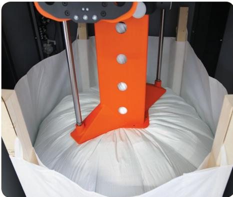
The inner bag is stretched and twisted at the same time. If needed, the procedure can be paused and resumed at a later stage.
