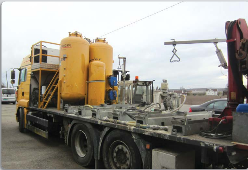
Pneumatic stretching arm on paint truck
