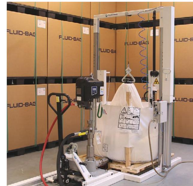
outlet pipe. In this case, the Discharge Roller stands on the floor. Normal pumps for offset ink can be used, piston pumps and diaphragm pumps being the most common. An adaptor is needed for an airtight connection to the pump (delivered with the Discharge Roller). Pump brand and model must be known to determine which adaptor to use.
