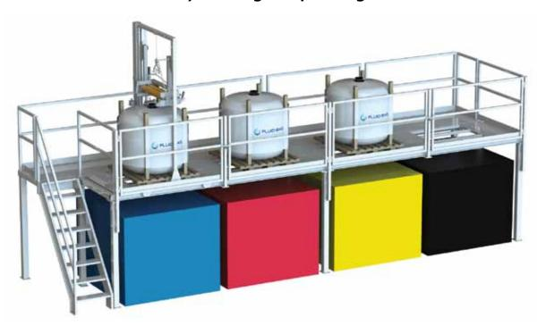
Fluid-Bag has developed a construction that enables a printer to use one or several Discharge Rollers for many mother tanks in a printing house. The purpose of the construction is to have a movable Discharge Roller on top of the mother tanks. The Discharge Roller moves on rails, hence it is called a rail system.
